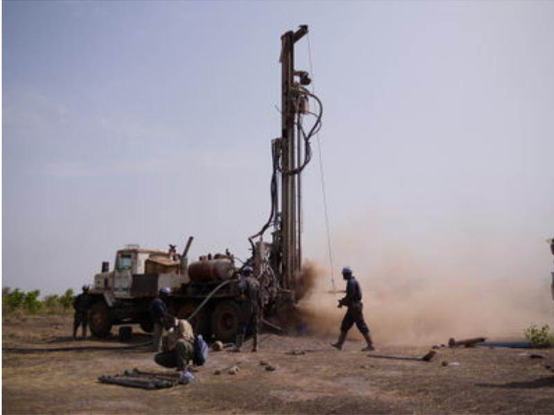
Drilling a water borehole with a rotary rig in Northern Region, Ghana. Photo credit: British Geological Survey.
