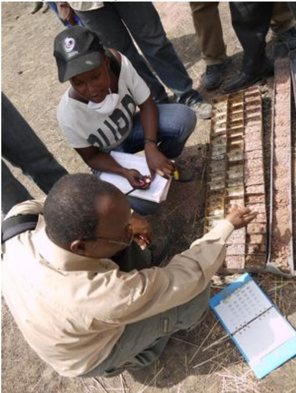
Rock cuttings from drilling laid out in sequence to be geologically logged by drilling supervisor. Photo credit: British Geological Survey.
