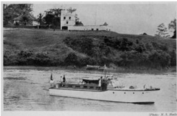
Geological Survey, British Territories In Borneo. Motor launch L'Aubaine built in 1952 for Geological Survey. Combined sea and river craft, 50 ft. long, range 500 miles, cruising speed 9 knots. Equipped for geological staff, and short expeditions into country. Photo: N. S. Haile. Plate XV.
