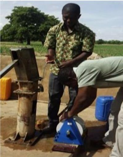
Dipping the water level in a borehole equipped with a hand pump. Image credit: Djibril Barry / WaterAid (2016)
