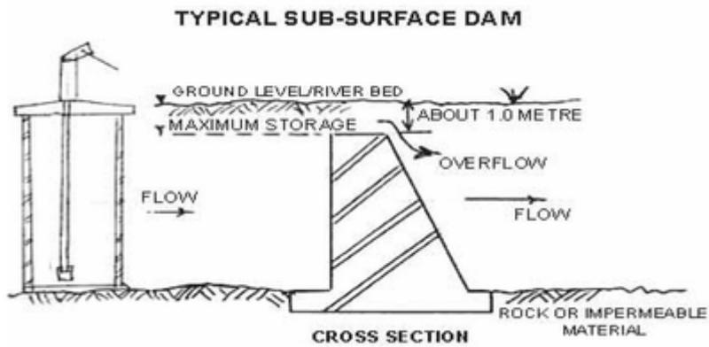
Subsurface groundwater dam profile. Image credit: [Onder and Yilmaz \(2005\)](#)
