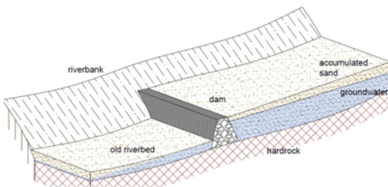
Schematic cross section of a typical sand storage dam. Image credit: [RAIN Foundation \(2011\)](#)
