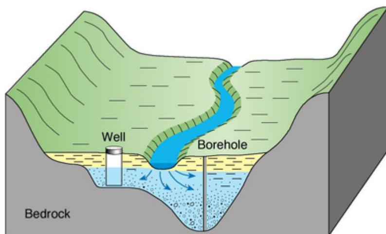
A schematic cross section of an alluvial aquifer in a river valley. Image credit: British Geological Survey
