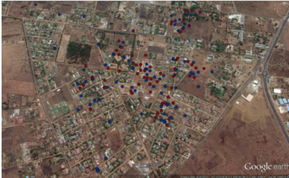
Figure 1: St. Bonaventure study site. Boreholes shown in blue, septic tanks in red (reproduced from Nkhuwa et al., 2015)
