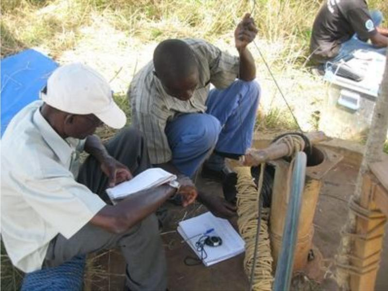
Carrying out a pumping test on a failed borehole in Uganda. Image credit: [Bonsor et al. 2013](#)
