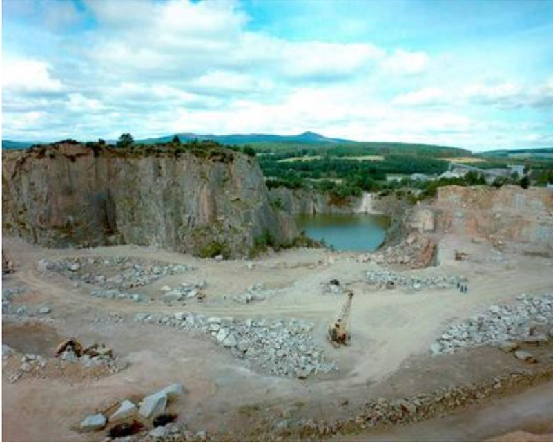
Kemnay Quarry, Aberdeenshire. The Kemnay granite is worked for aggregate, dimension stone and cladding. In the background is the granite mass of Bennachie (D 4337). P000206.
