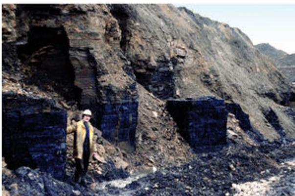
Pillars of coal, the roof supports left behind in old, shallow mine workings, re-appearing in modern excavations at the Langley opencast site, Northumberland [NZ 200 469]. (P711118).
