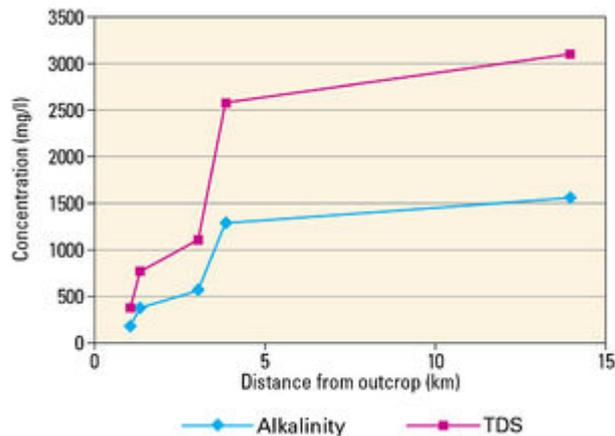
Alkalinity and total dissolved solids evolution down dip in the Old Coal Horizon (after Ineson, 1967). P859275.
