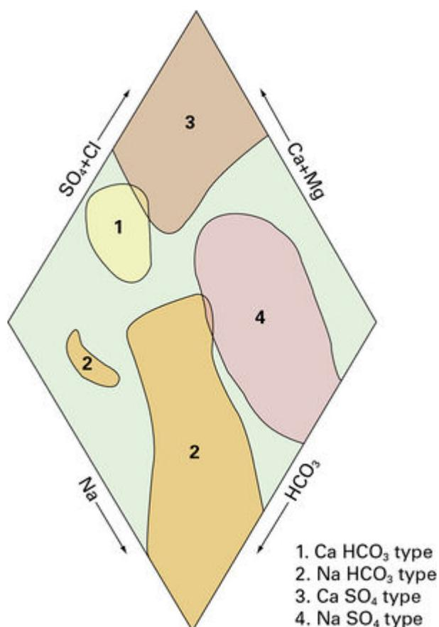
Piper diagram showing the distribution of the four main groundwater types in the South Wales Coal Measures Group (after Ineson, 1967). P859276.
