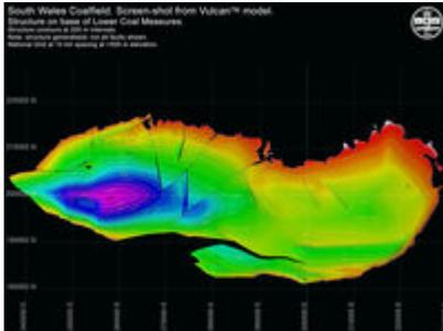
Screen shot showing the structure on the base of the South Wales Lower Coal Measures Formation with contours at 200 m intervals: dark purple -2500 m OD; green -1000 m OD; orange 0m OD. P859292.
