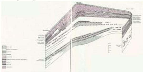
Figure 3 Generalised ribbon diagram showing lateral variations in the Carneddau Group and Snowdon/Crafnant Volcanic groups between Dolwyddelan and Betws-y-Coed. Intrusions omitted.
