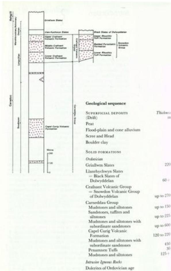
Figure 2 Generalised vertical section showing the relationships of the broad lithostratigraphical divisions to the Caradoc Shelly stages.
