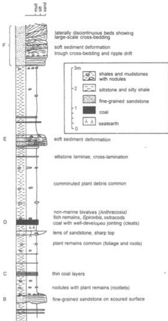
Figure 10.3 (a) Simplified sedimentary log of the sequence exposed in Bradgate Brickyard quarry.
