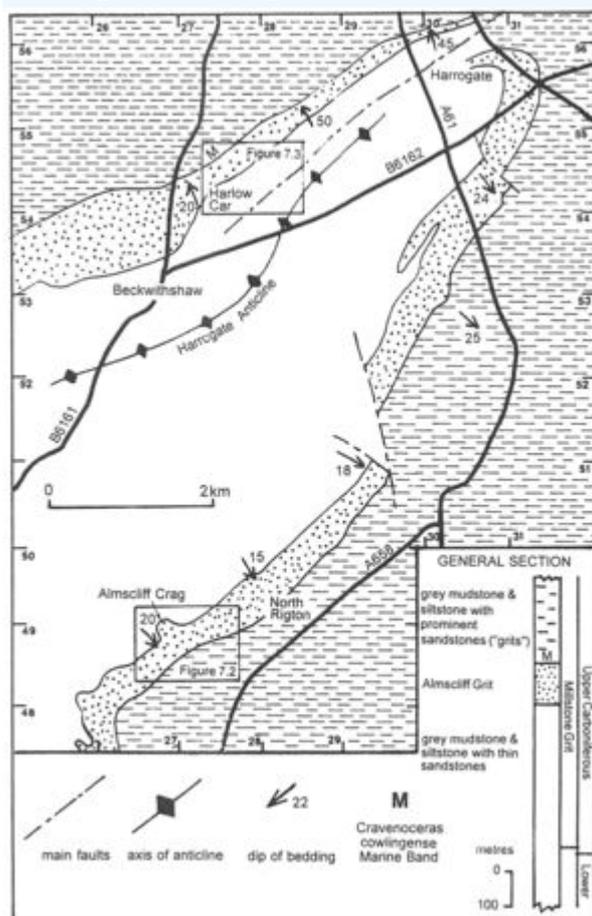
Figure 7.1 Outline geology of the Harrogate Anticline, and main road network.
