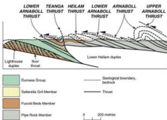
Cross-section through the Heilam area, after Butler (2009), extending from the Lighthouse duplex in the WNW (left) to Loch Hope in the ESE (right).
