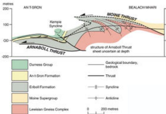
Cross-section of the Kempie area, after Butler (2009), extending from An t-Sròn in the WNW to Bealach Mhari in the ESE.
