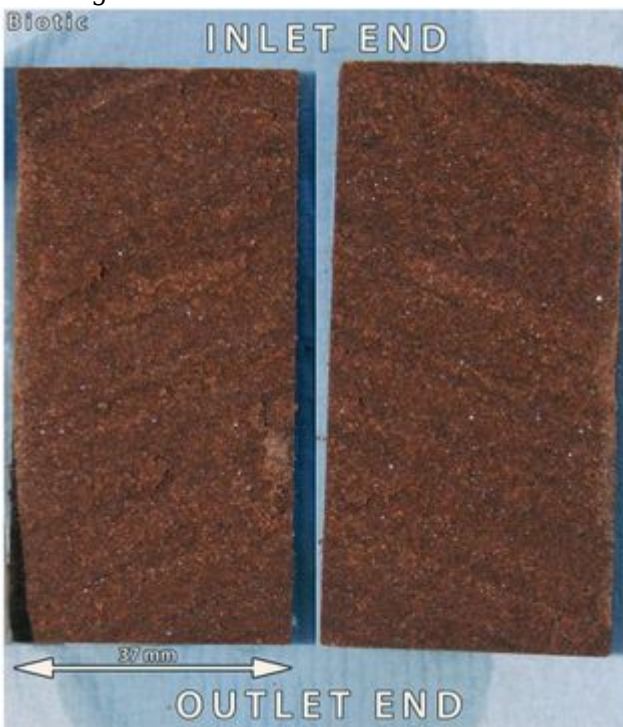
• Plate 16 Biotic test plug freshly fractured, showing the strongly defined bedding structures. The grey staining observed on the outside of the plug has not penetrated the plug interior.
