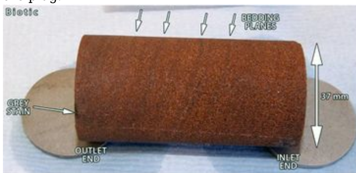
Plate 14 Test plug and end frits after removal of the outer casing, showing the patch of grey stain on the outside at the outlet end. Bedding planes are indicated.
