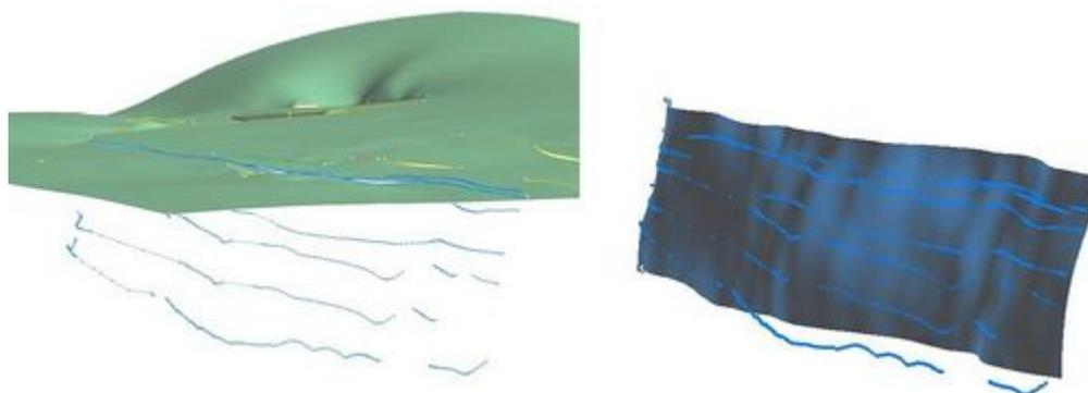
**Figure 7** Example from the Northumberland-Solway Model showing the construction of a fault surface (the Closehouse-Lunedale fault) from fault sticks (right image in blue) and the interaction of the fault with the Permo-Trias surface prior to faulting (in green) from Terrington *et al* (2013)<sup>[3]</sup>.
