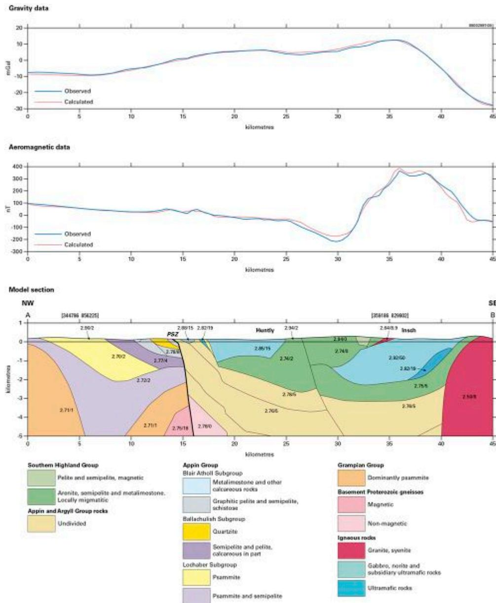
**Figure 9** Part of a full-crust modelled section across the Huntly and Insch plutons. Location shown in Figure 7. The numbers cited inside the polygons indicate the bedrock density and magnetic susceptibility values used in the model.
