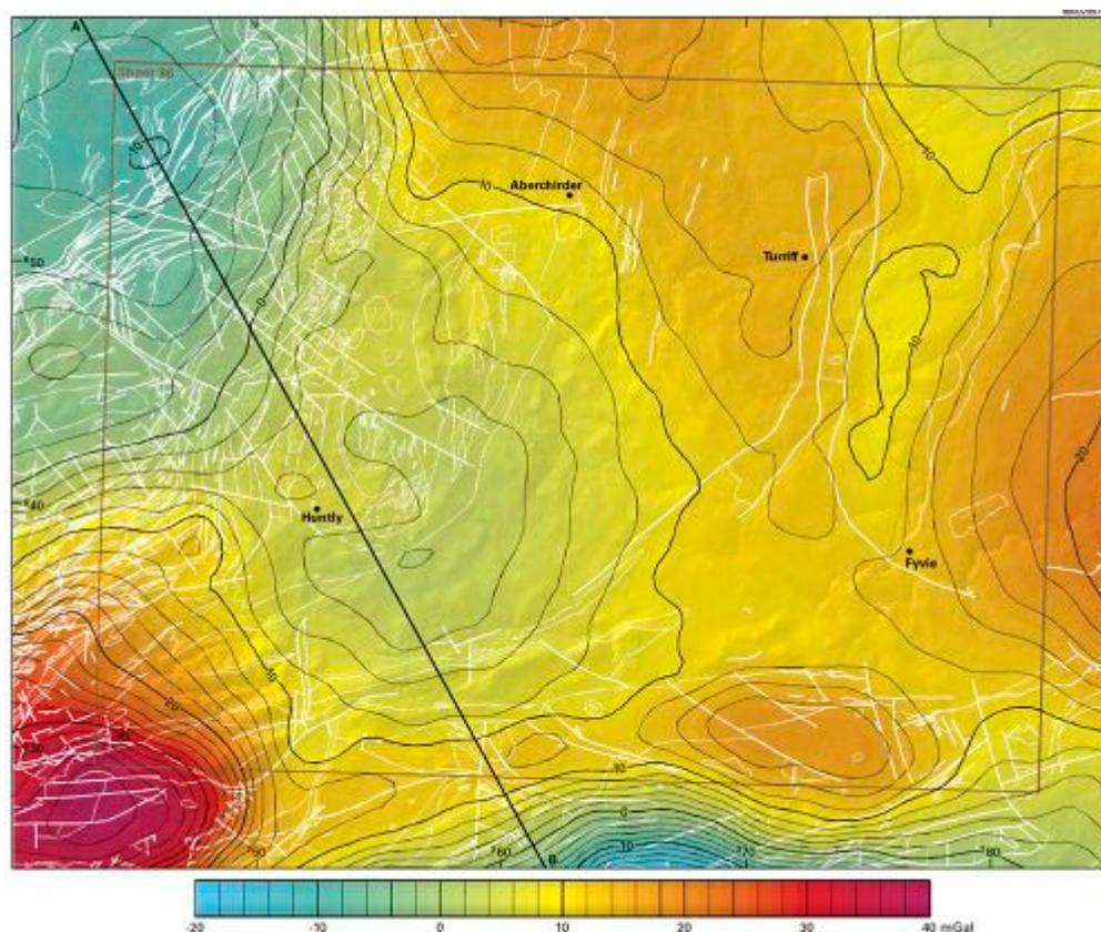
**Figure 7** Bouguer gravity anomalies in the Huntly and Turriff districts. Values based on a reduction density of  $2.75 \text{ Mgm}^{-3}$ . The underlying white lines relate to the generalised bedrock geology, based on the 1:250 000 geological map.
