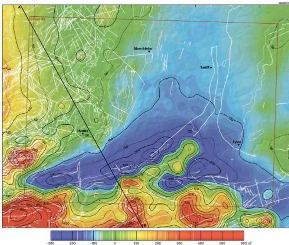
**Figure 8** Total field magnetic anomaly in the Huntly and Turriff districts. Contours based on data collected at 305 m above ground level on east-west flight lines 2 km apart. The underlying white lines relate to the generalised bedrock geology, based on the 1:250 000 geological map.
