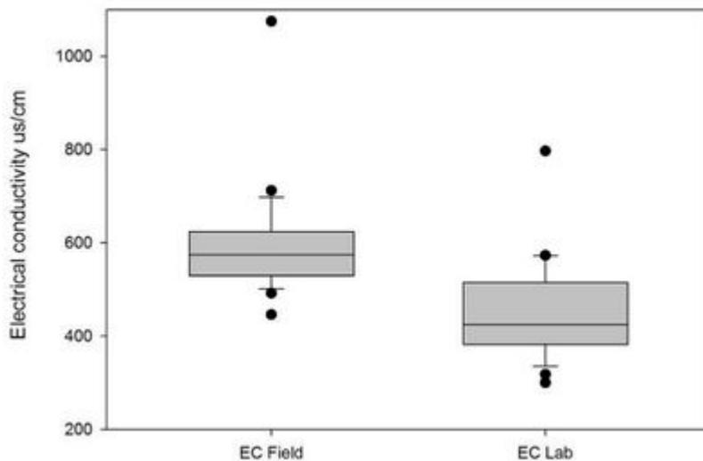
**Figure 4-4** Electrical conductivity field versus laboratory (n= 24).
