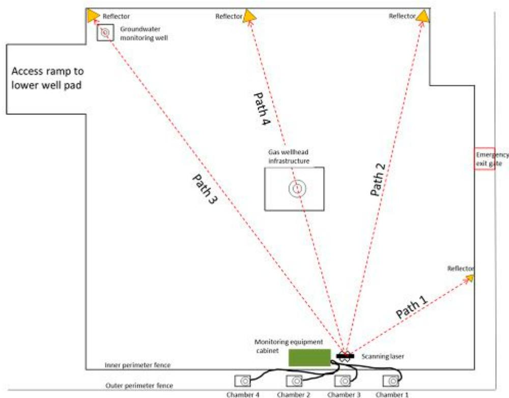
**Figure 122** Layout of automated flux chambers and scanning CH<sub>4</sub> laser at KM8.
