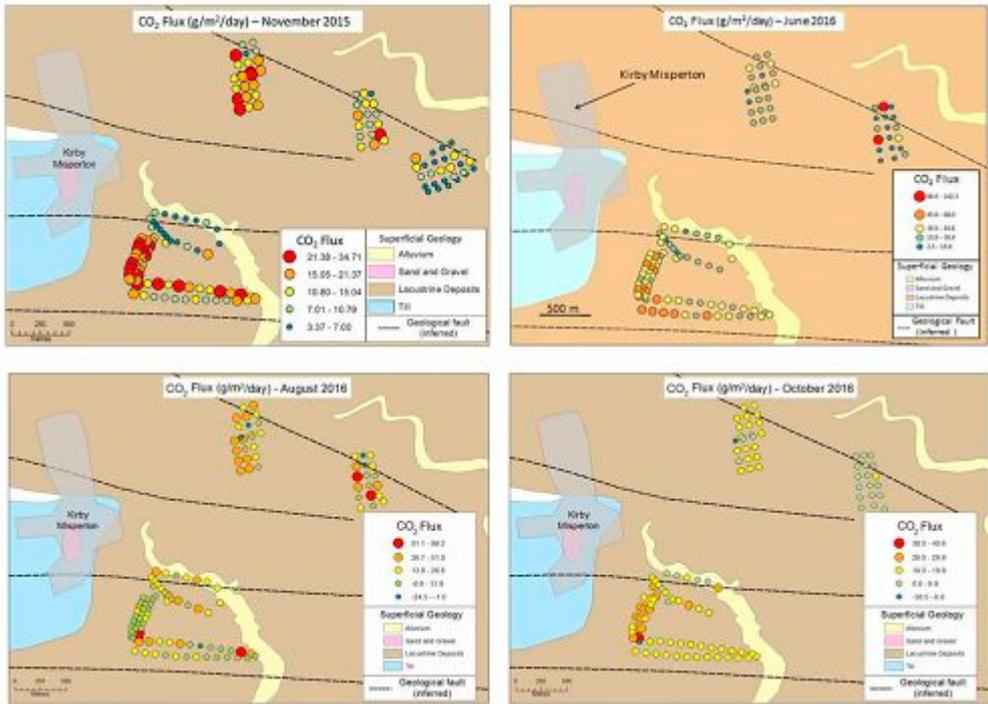
**Figure 116** Spatial plots of CO<sub>2</sub> flux from the soil for the different surveys.
