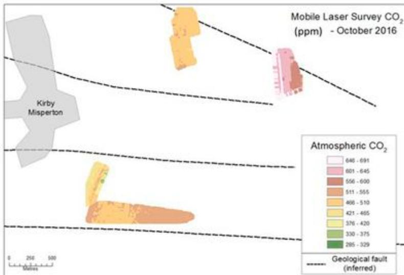
**Figure 120** An example of mobile open path laser data for CO<sub>2</sub> from October 2016.
