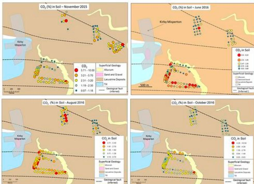
**Figure 115** Spatial plots of CO<sub>2</sub> in soil gas for the different surveys.
