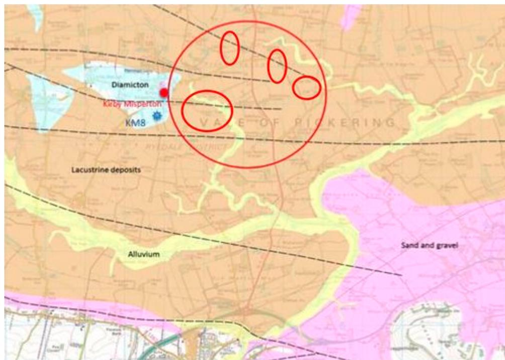
**Figure 111** Soil gas study area to the east of Kirby Misperton within the red circle. Includes mapping data licensed from Ordnance Survey. © Crown Copyright and/or database right 2017. Licence number 100021290 EUL.
