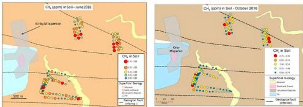
**Figure 117** Methane concentrations in soil gas for June and October 2016.
