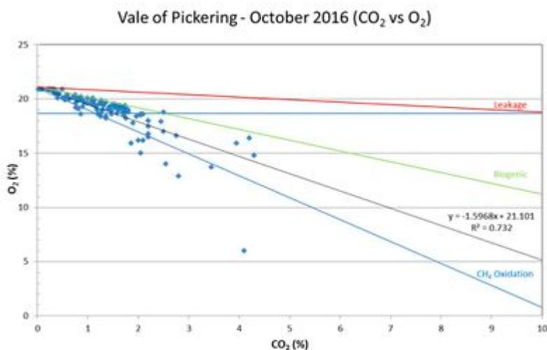
**Figure 121** CO<sub>2</sub>/O<sub>2</sub> ratio plot for soil gas data from October 2016.
