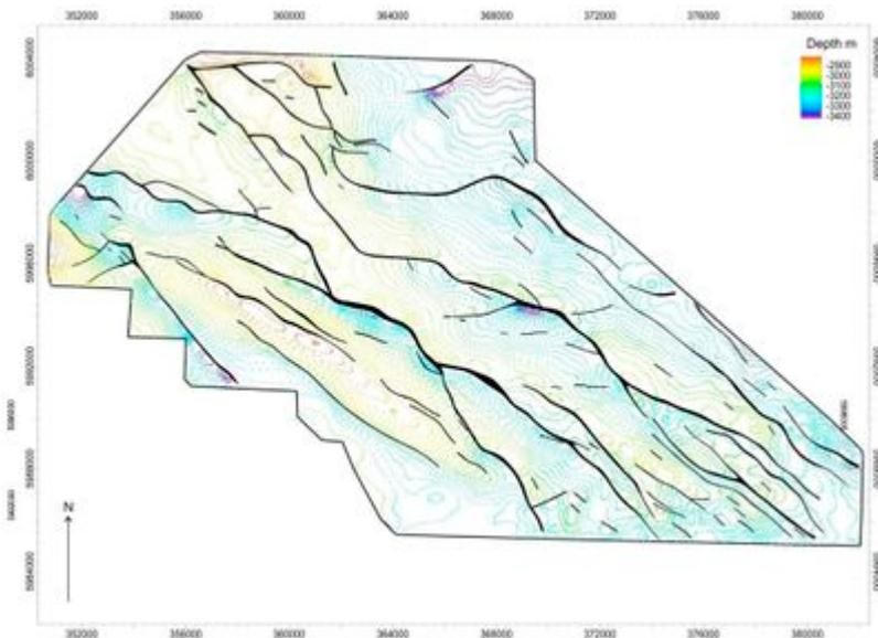
Figure 3 Structure at Top Leman Sandstone. Digitised from Ketter (1991a)<sup>[1]</sup> and imported to PETREL. Image from PETREL (fault polygons and contour points).
