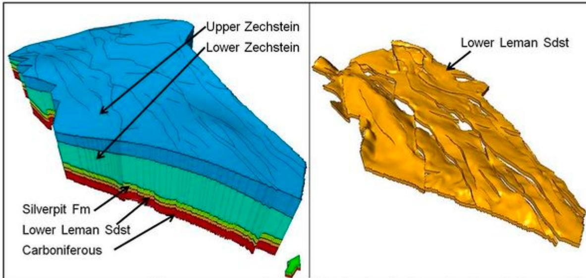
Figure 5 3D perspective view of the Ravenspurtn 3D geological model. Left: with overburden, Right: with overburden removed.
