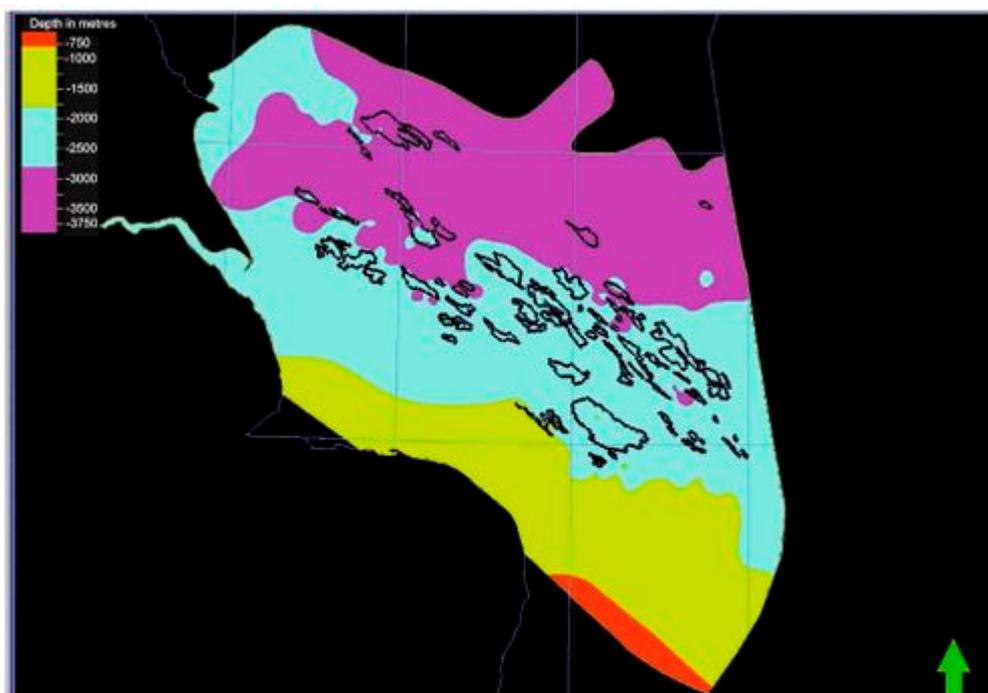
Figure 11 Depth to top Lower Leman Sandstone (m).
