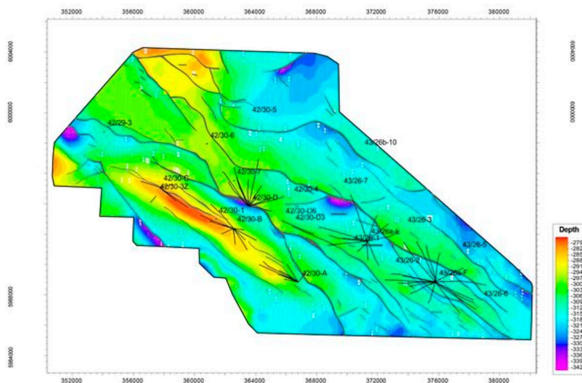
Figure 4 Location of the 80 wells in the model that penetrate the top Lower Lemman Sandstone Formation surface (coloured by Z values). Digital well data from the CDA website, <https://www.ukoilandgasdata.com/>
