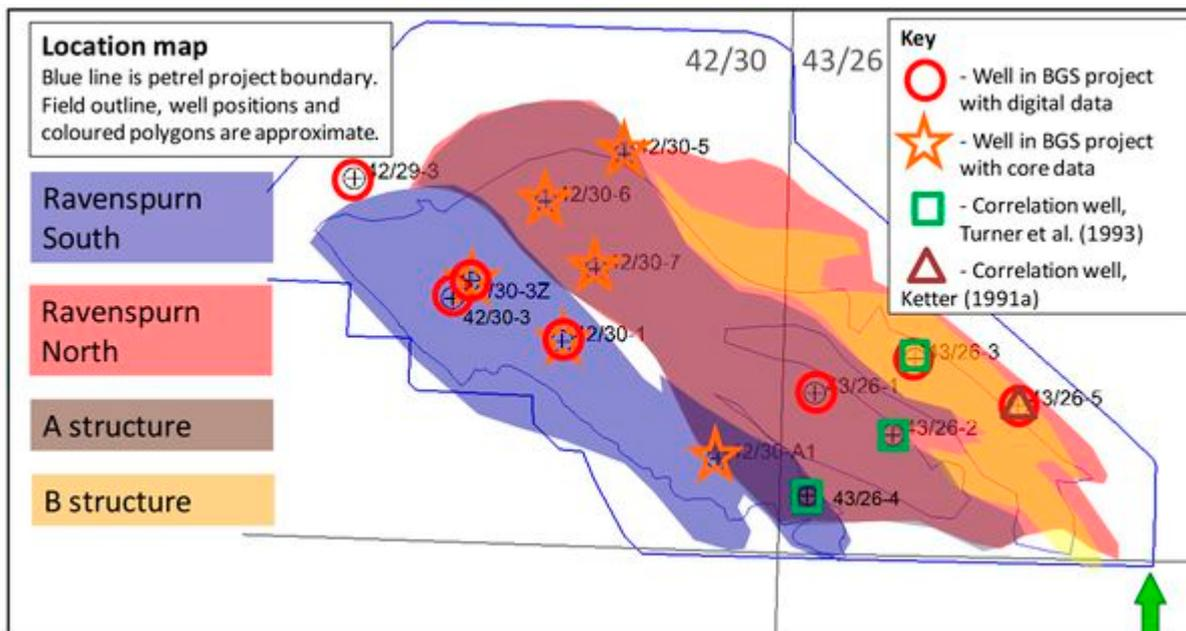
Figure 6 Map of Ravenspurn structure, with sketched shapes overlain to indicate structural regions referred to in the text and the wells with data available. Well and hydrocarbon field locations from <http://data-ogauthority.opendata.arcgis.com/>
