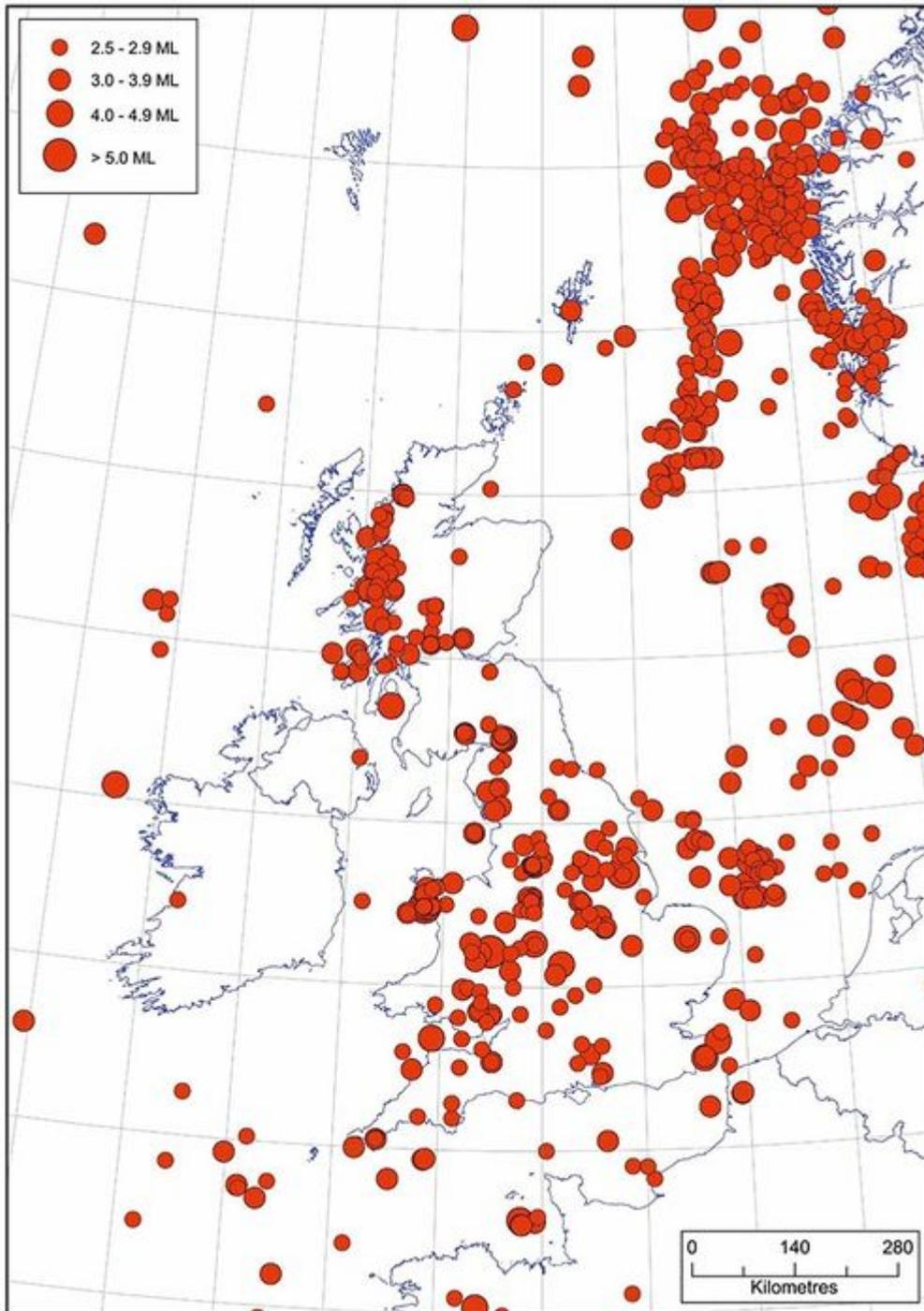
**Figure 3** Epicentres of earthquakes with magnitudes of 2.5 ML and above, in the period 1979 to 2017.
