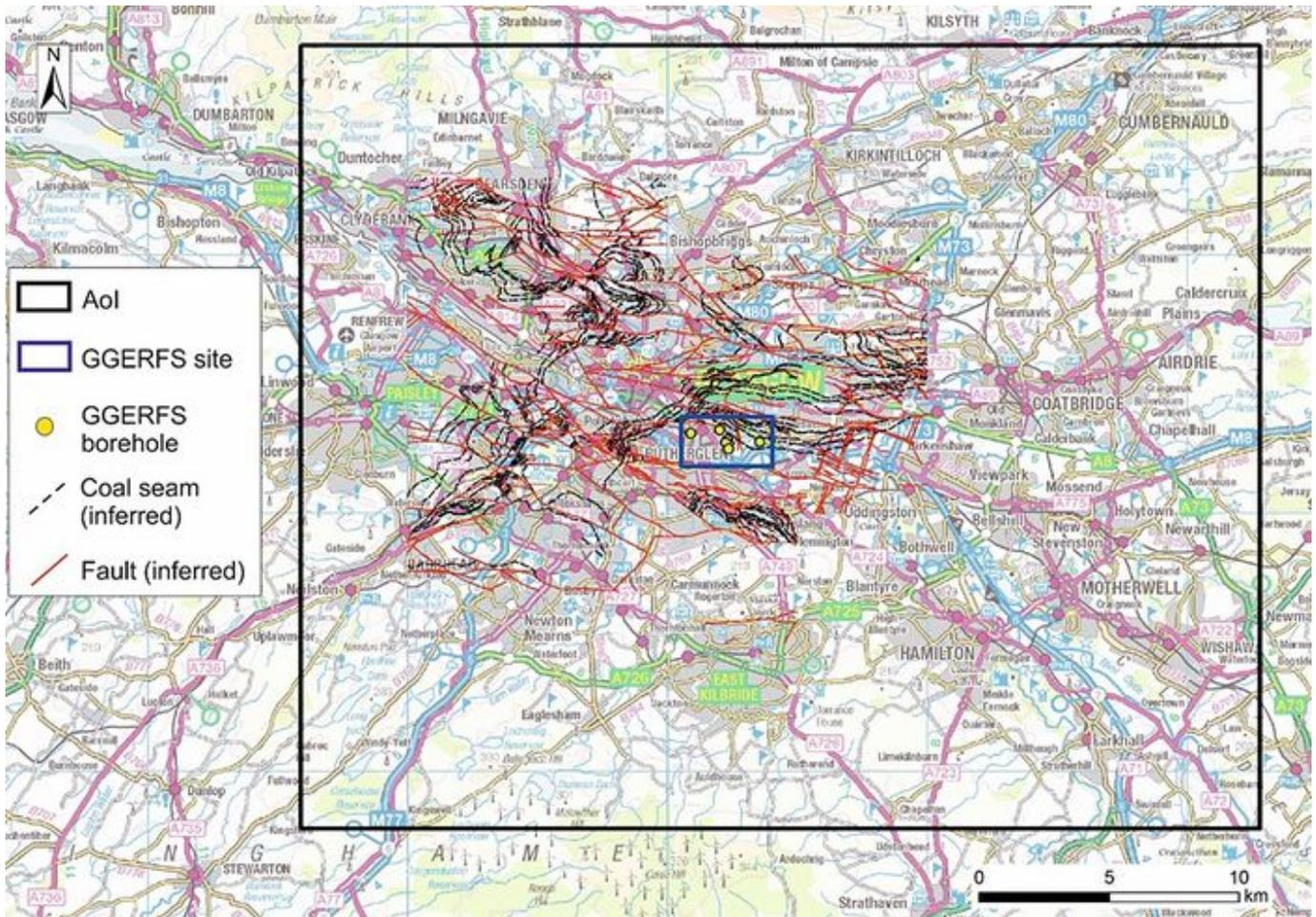
**Figure 1** GGERFS site and the extent of the AoI processed with ERS, ENVISAT and S-1 SAR imagery. Coal seam and fault locations are shown for to the central part of Glasgow only. Contains Ordnance Survey data © Crown copyright and database right 2018, license number 100021290 EUL. Contains British Geological Survey materials © UKRI 2019.
