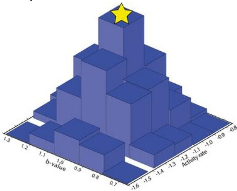
**Figure 3** Probability density function for the activity rate and the b-value of the source zone EC9M of the UK source model. The star indicates the most likely value for the
