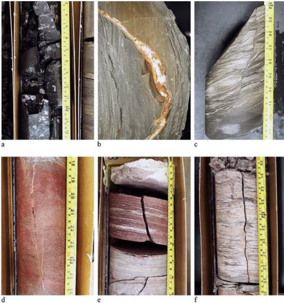
Figure 11 Character of discontinuities in core GGC01.
