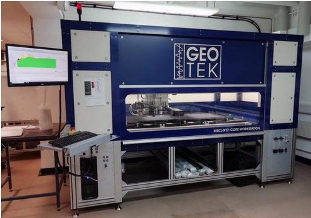
**Figure 18** X-ray fluorescence scanner (Geotek, MSCL-XYZ XRF).
