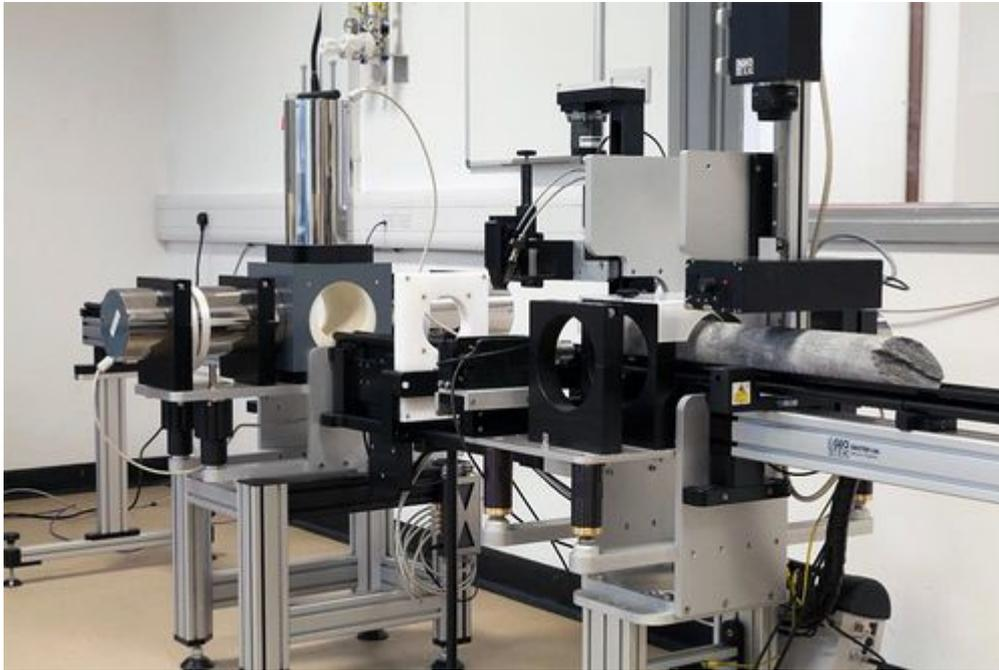
**Figure 17** Multi-sensor core logging scanner (Geotek MSCL-S).
