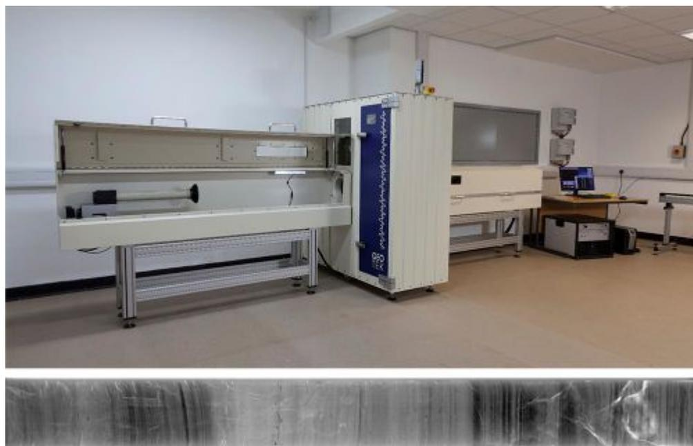
**Figure 16** MSCL-RXCT core scanner and example 2D X-ray radiograph (Geotek MSCL — RXCT).
