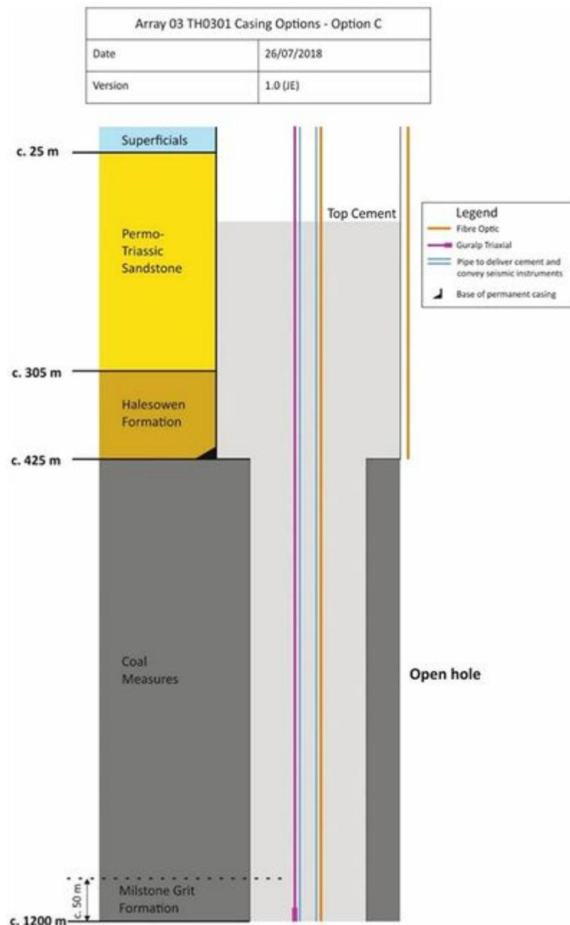
**Figure 19** Array 3 Borehole construction/casing options and prognosis.
