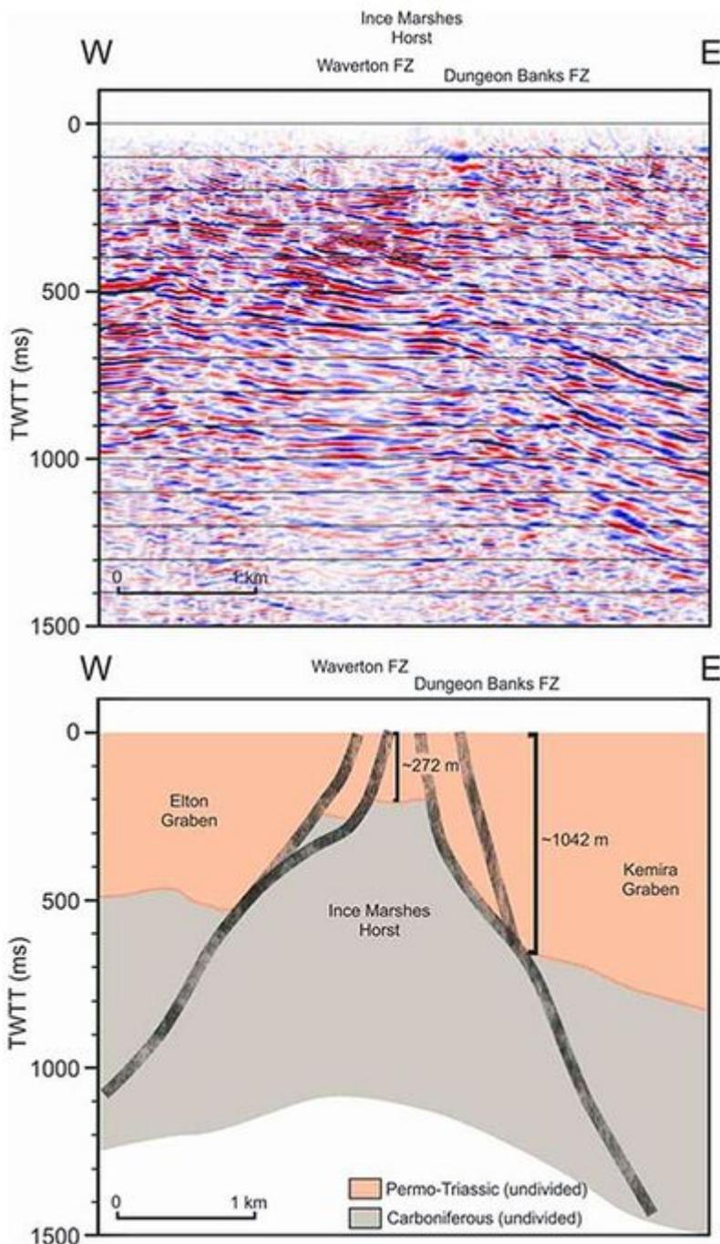
**Figure 6** General structure of the Ince Marshes area, based on interpretation of seismic-reflection line SC-83-128V, illustrating the Ince Marshes horst structure defined by the Waverton fault zone to the west and Dungeon Banks fault zone to the east. FZ = fault zone. (Seismic data courtesy of UKOGL).
