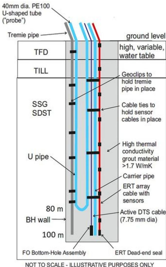
**Figure 12** Schematic well design for Thermal Response Test (TRT) well showing positioning of DTS and ERT cables on outside of 40 mm diameter PE100 U-shaped tube.
