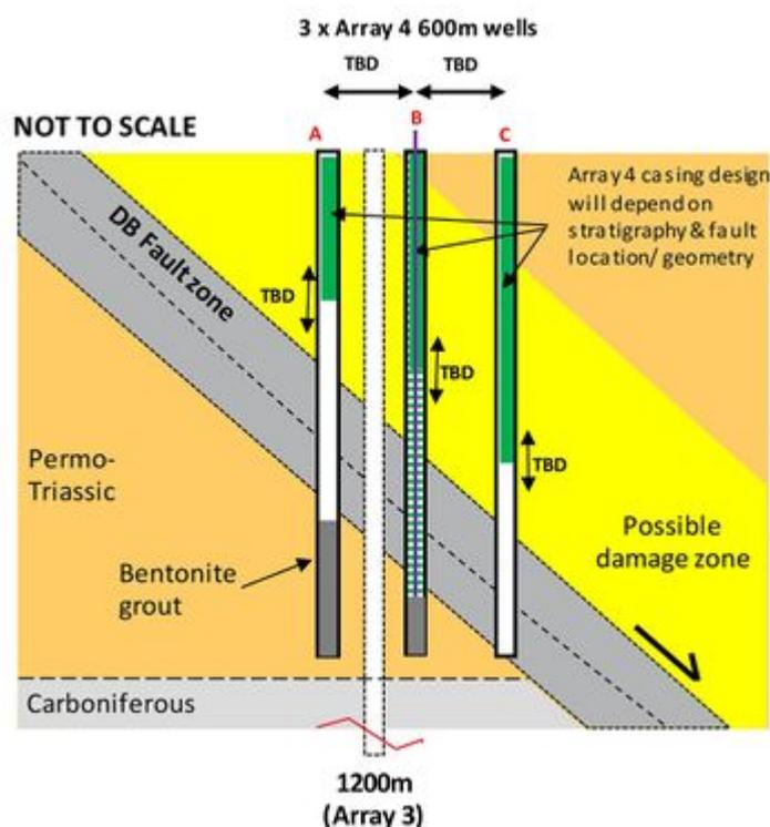
**Figure 13** Design concept for 3 x 600 m Array 4 boreholes: the middle 600m borehole is installed with a well casing/screen instrumented with DTS & ERT cables to support online monitoring of fluid flow. Note that the 1200 m array 3 borehole is located out of the plane of section.
