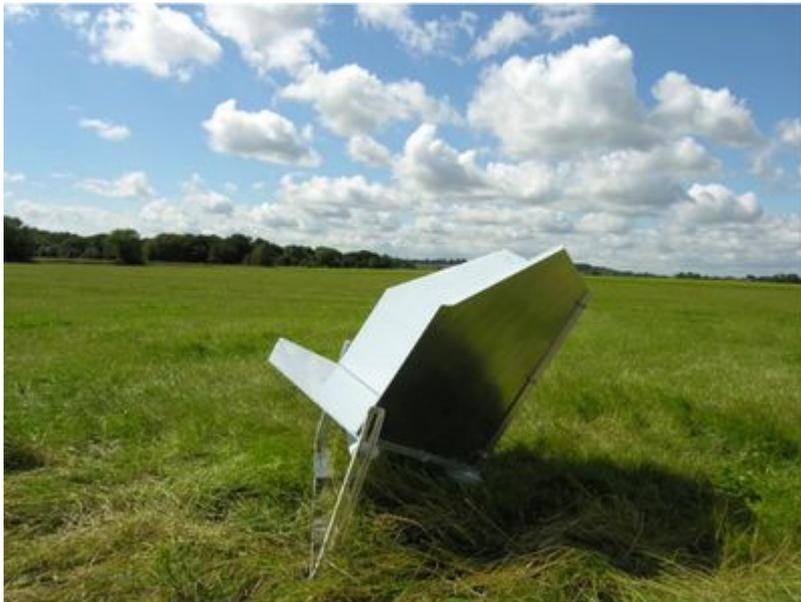
**Figure 14** Passive InSAR reflector.
