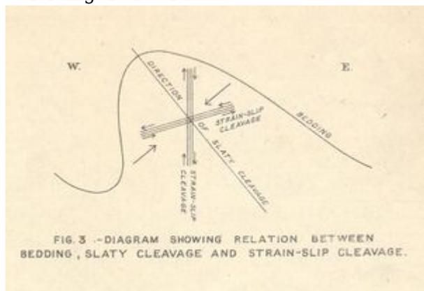
Diagram showing relation between bedding, slaty cleavage and strain-slip cleavage. P519815.
