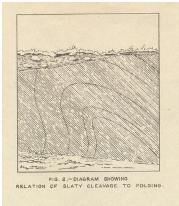
Diagram showing relation of slaty cleavage to folding. P519814.
