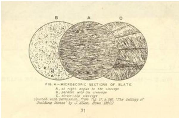
Microscopic sections of slate. A. at right angles to the cleavage. B. parallel with the cleavage, C. strain-slip cleavage (Quoted with permission from fig. 17 p.280 'The geology of building stones' by J. Allen Howe, 1910. P519816.
