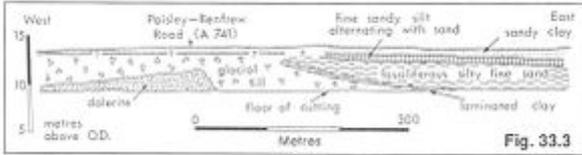
Figure 33.3. Composite W-E section formerly exposed at Junction 27 on the M8 motorway near Paisley, showing a roche moutonnee (of dolerite) overlain by till which, in turn, is overlain by laminated clay and fossiliferous marine sediments (Clyde Beds).
