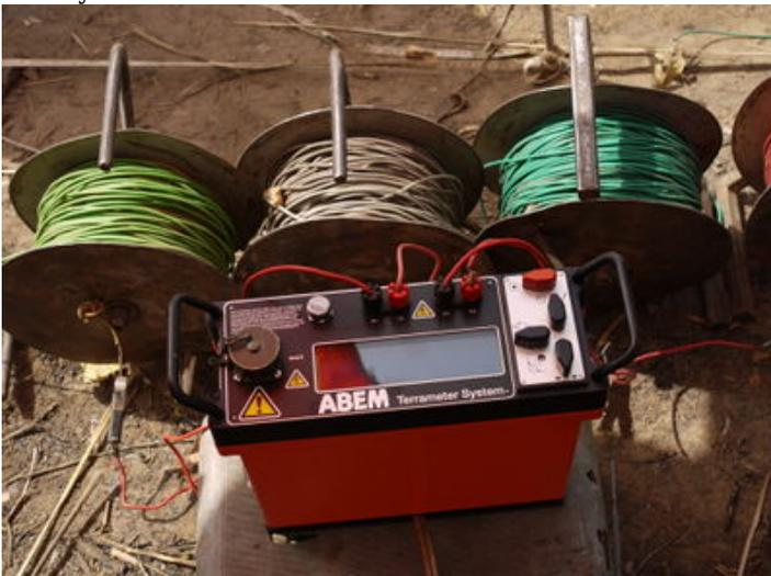
Resistivity surveying equipment for geophysical surveying. Photo credit: British Geological Survey.
