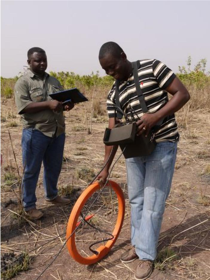
Geophysical surveying for water borehole siting in Northern Ghana, using EM34. Photo credit: British Geological Survey.
