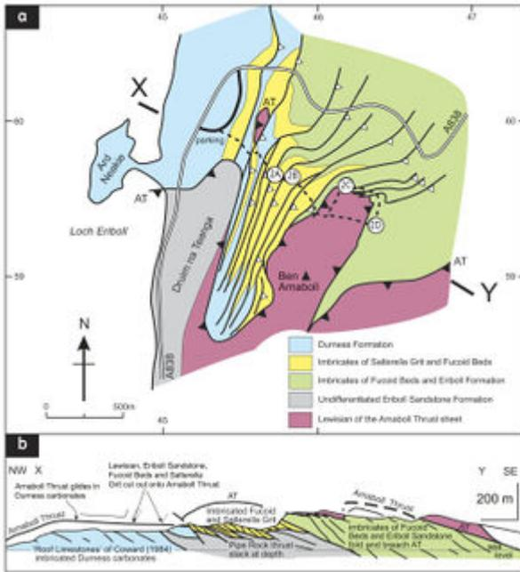
Fig. 11.7 Simplified geological map (a) and cross-section (b) of the Arnaboll hill area. Modified after Coward, 1984
